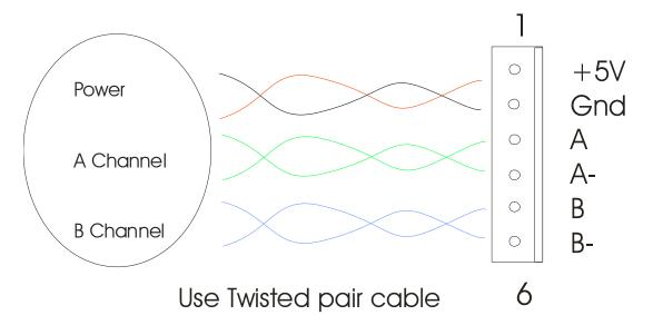
**Note**: Diagram shown for a differential encoder. For a single ended encoder, use just one connection per channel. Use (stranded) twisted pair cable for encoder wire. Use shielded wire if available. Connect the shield on *one end only* to avoid current flowing in shield.
