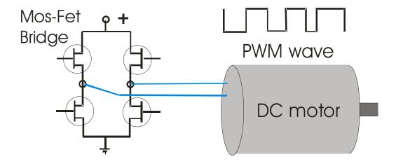
The Viper drive uses a Mos-Fet or an IGBT bridge to drive the servo motor. The signal is Pulse Width Modulation or PWM with a frequency of 20,000 HZ
