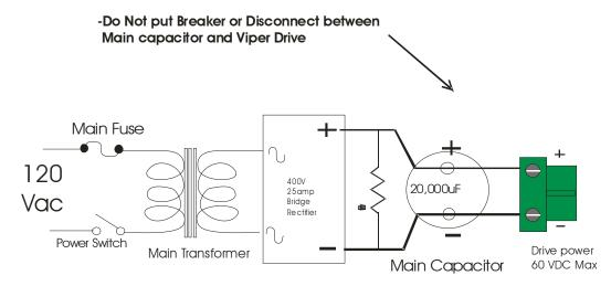
The Maximum DC powersupply voltage to the Viper 60 is 60 volts.
